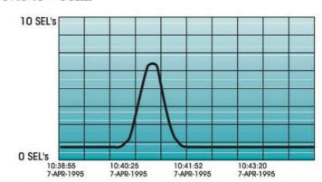
The above trace shows a typical increase in trauma placed on a pump as the supply of product was momentarily shut off.
